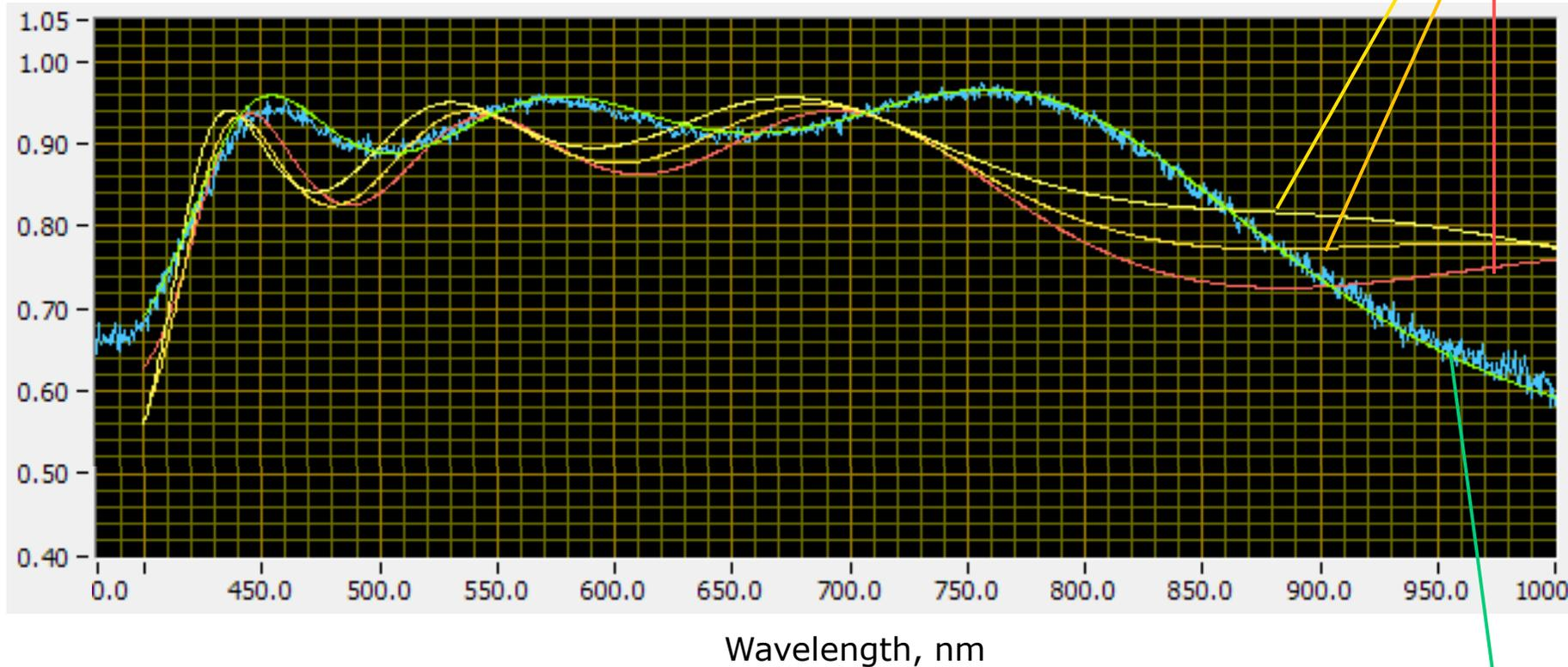
Simulated 80% of target thickness
