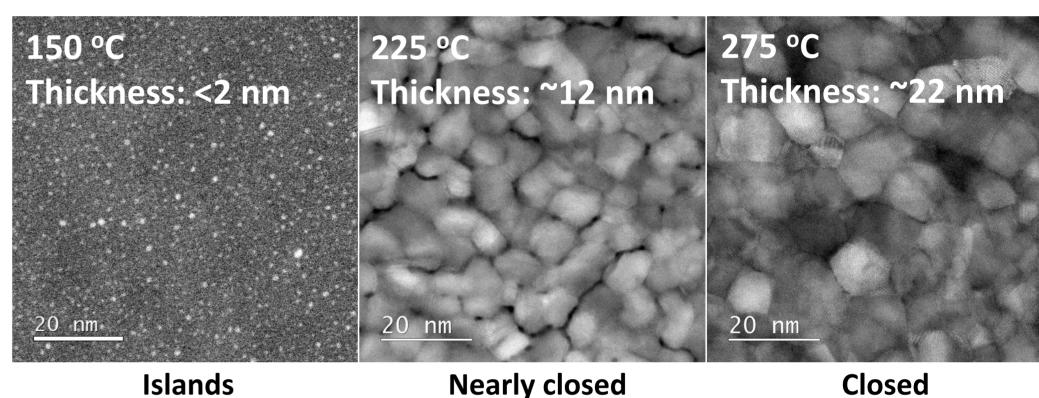
In-situ spectroscopic ellipsometry and scanning electron microscopy of
