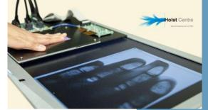
Flexible electronics: -Thin (10nm - 10µm) layers with functionality over large-area
