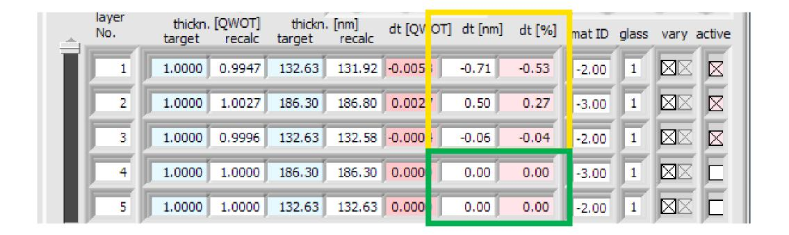
Small thickness errors can be alleviated by reoptimization of optical stack. Thickness of the following layers will be recalculated to maintain optical function of the layer stack.
