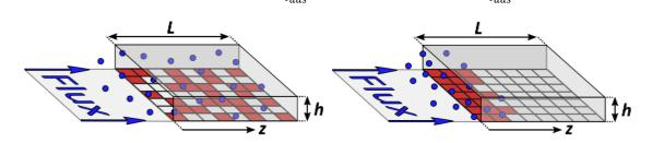
Figure 3: Illustration of reaction-limited growth (left) and diffusion-limited growth (right).
