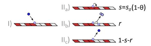
Figure 2: Illustration of the modeled interaction between gas-phase reactant species (blue circles) and the surface during (plasma) ALD, where the squares represent empty (white) and occupied (red) adsorption sites. When a reactant molecule or atom hits the surface (I), it can adsorb at an empty adsorption site ( $II_a$ ), recombine with another atom at the surface ( $II_b$ ) or reflect ( $II_c$ ). Only adsorption ( $II_a$ ) leads to an increase in surface coverage.
