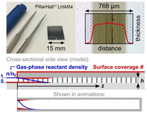
Figure 4: Pictures of PillarHall<sup>TM</sup> horizontal trench structures (top) supplied by VTT that we used in our experiments, where the silicon membrane is removed and the deposited film is visible. The schematic cross section of the structure (middle) shows the gas-phase reactant density (blue line) and surface coverage (red outline) in the same way as in the animations provided in this blog post (bottom).
